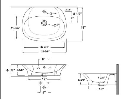
Dimensions of fixture are nominal and may vary within the range of tolerances established by ASME Standard A112.19.2.2018 Dimensions and specifications subject to change without notice.
